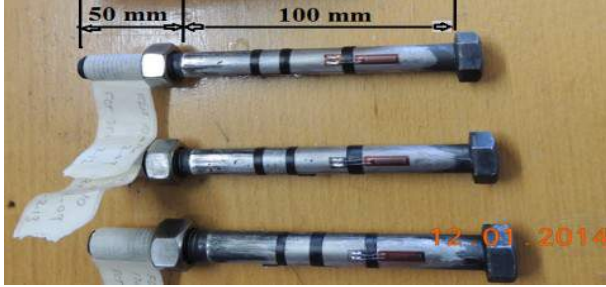
Fig. 3. Length of testing bolts
