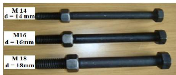
Fig. 2. Different diameters of testing bolts
