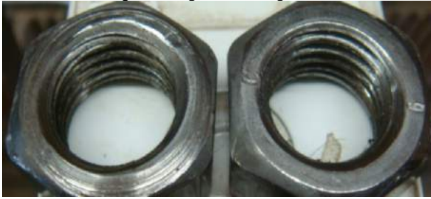
Fig. 4 Friction scratches on nut surface
